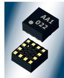
Kionix's newest 2x2x0.9mm robust accelerometer maintains power as low as 10uA while offering a wide variety of embedded algorithms, including tap detection, orientation detection, activity monitoring, and user-configurable motion wake-up.
