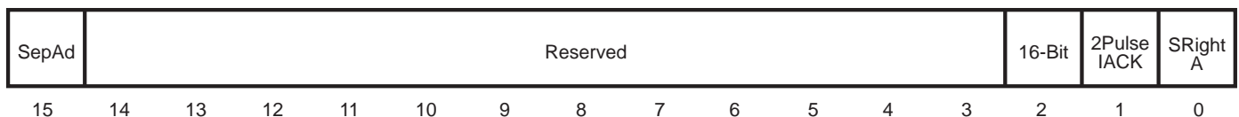
Figure 2-7. The USC's Bus Configuration Register (BCR)
